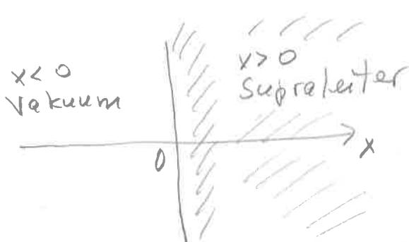
$$\frac{\partial^2 \vec{B}}{\partial x^2} = \frac{4\pi n_s e^2}{mc^2} \vec{B} \quad (x > 0)$$
